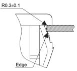
Process the above-mentioned R on the mounting hole side of panel, or be sure that the Play R is on the operation side of panel when using.
