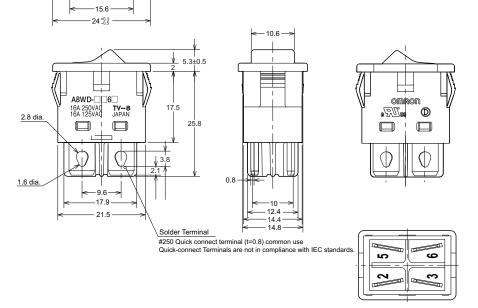
Note: Unless otherwise specified, a tolerance of ±0.3 mm applies to all dimensions.
