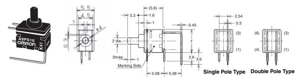
**Note:** Unless otherwise specified, a tolerance of  $\pm 0.4$  mm applies to all dimensions.
