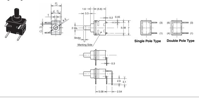
Note: Unless otherwise specified, a tolerance of  $\pm 0.4$  mm applies to all dimensions.
