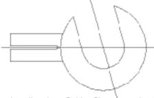
Used to install various Solder Sleeve termination devices, such as shield terminators, wire splices, and coaxial cable terminators. Also used for installing Soldertacts® contacts and for heating Mini-Seal® splice sealing sleeves and small-diameter heat-shrinkable tubing.
