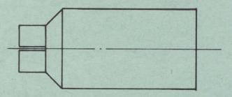
Provides a larger volume of heated air at a lower temperature than is obtained with no tip. Used to install heat-shrinkable molded parts and tubing without hot-spot overheating.
