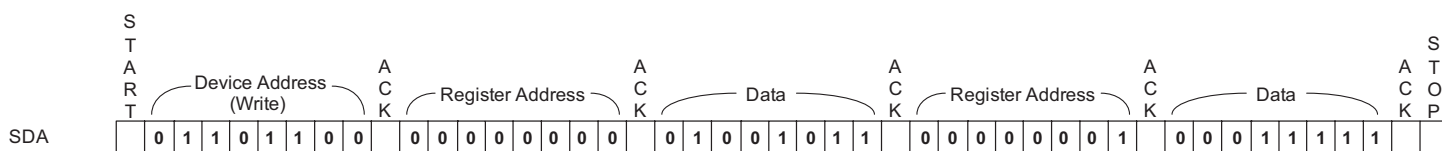
Figure 5: I 2 C Transfer Protocol for Example 1.
