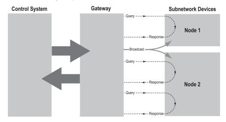
In Master Mode, Anybus Configuration Manager comes preloaded with most commonly used Modbus RTU commands, which can conveniently be reached by right-clicking on a node in the Anybus Configuration Manager and selecting "Insert New Command". Note however that this does not in any way prevent other protocols based on the same query-response message-scheme to be implemented.
