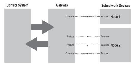
In the figure above, the gateway 'consumes' data that is 'produced' by a node on the subnetwork. This 'consumed' data can then be accessed from the higher level network. This also works the other way around; the data received from the higher level network is used to 'produce' a message on the subnetwork to be 'consumed' by a node.
