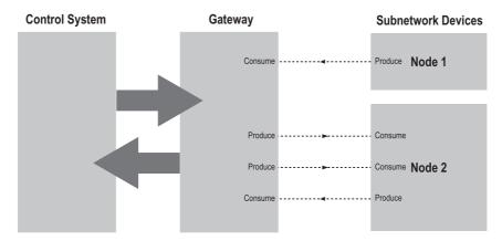
In the figure above, the Anybus Communicator 'consumes' data 'produced' by a node on the sub-network. This 'consumed' data can then be accessed from the higher level network. This also works the other way around; the data received from the higher level network is used to 'produce' a message on the sub-network, for 'consumtion' by a node.
