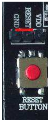
Figure 9: Jumper setting for low effective RESET
