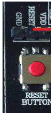
Figure 8: Jumper setting for high effective RESET
