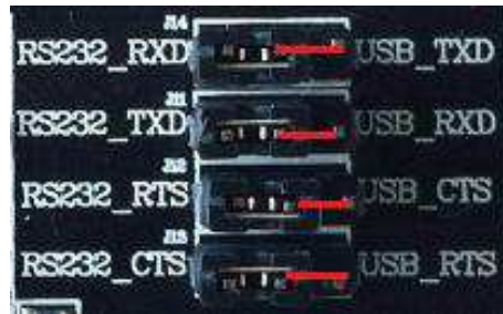
Figure 5: USB to serial jumper connect
