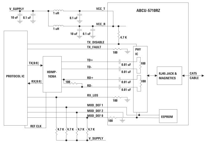
Figure 4. Typical Application Configuration for ABCU-5710RZ
