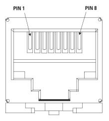
Figure 3. MDI (RJ 45 Jack) Pin Assignment
