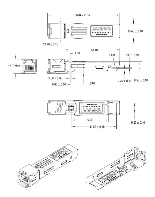
Figure 7a. Module Drawing
