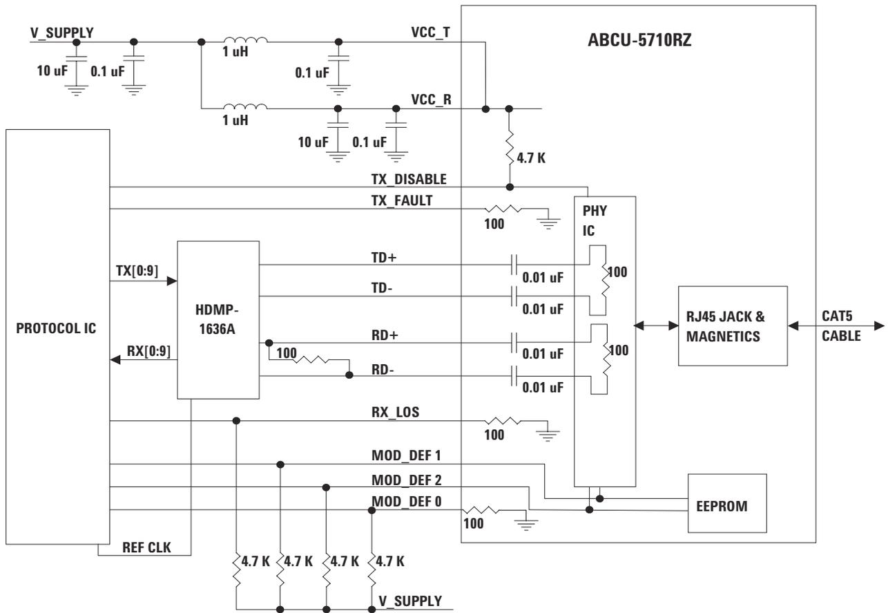
Figure 4. Typical Application Configuration for ABCU-5710RZ
