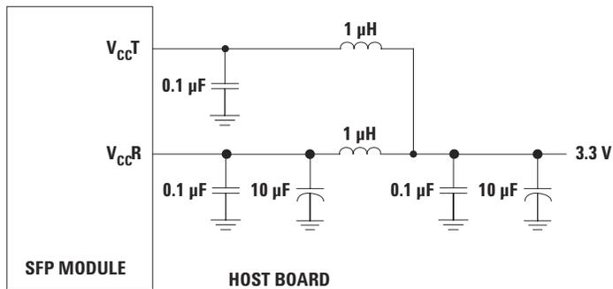
Note: Inductors must have less than 1ohm series resistance per MSA
