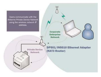
The Ethernet Adapter from Quatech includes a fully functional Network Address Translation (NAT) router. When coupled with the built-in DHCP server on the Ethernet port the most powerful Ethernet adapter in the M2M market comes to life. Your Ethernet device needs no special security settings, IP configuration or proprietary protocols. If it supports DHCP or Static IP addressing you can quickly connect to the most advanced Enterprise class networks without changing your platform.
