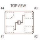
• #1,#3 : Crystal terminal / #2,#4 : Connected to cover (Please connect it with GND.)
