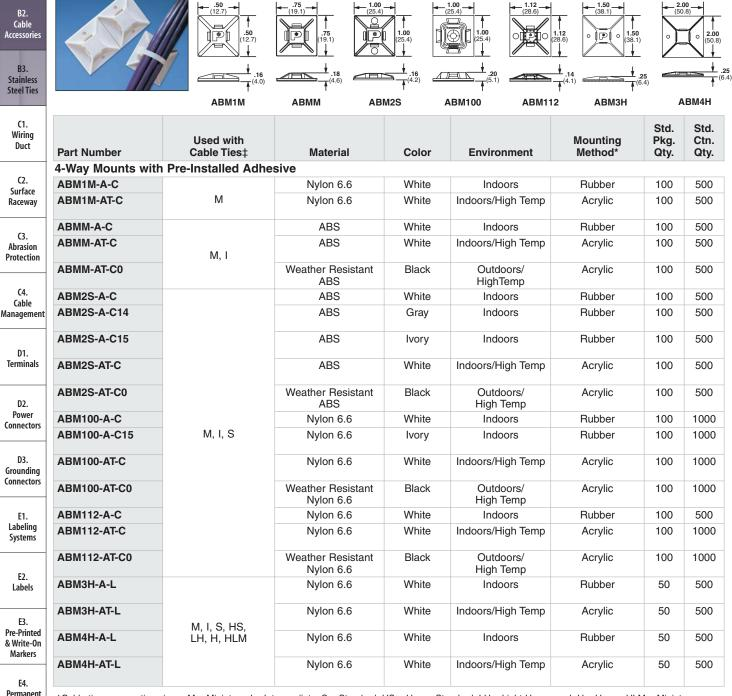
‡Cable tie cross section sizes: M = Miniature, I = Intermediate, S = Standard, HS = Heavy-Standard, LH = Light-Heavy, and H = Heavy, HLM = Miniature Tak-Ty® Hook & Loop Ties.
