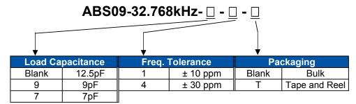
\*Contact ABRACON for non-standard load capacitance
