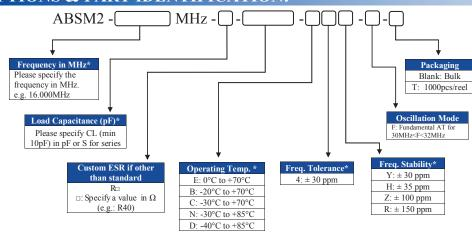
\*Frequency, Load Capacitance, Frequency tolerance and stability is subject to availability. Please contact Abracon for each option for availability.
