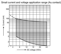
3) When selecting a contact type of a snap-action switch to be used for low-level load switching, the following should be noted. Silver contacts' surfaces are prone to be oxidized and form a sulfide film. The switch operates with no problems at the
