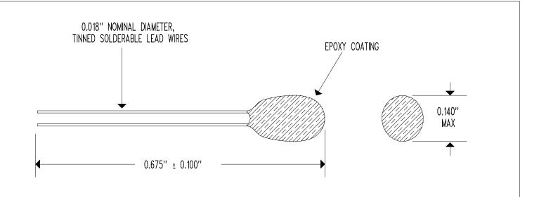
RESISTANCE @  $+25^{\circ}$ C = 10,000  $\Omega$  ± 1% RESISTANCE/TEMPERATURE CURVE = "E1" BETA " $\beta$ " (+25 TO +85°C) = 3,435°K NOMINAL DISSIPATION CONSTANT = 2 mW/°C NOMINAL THERMAL TIME CONSTANT = 15 SECONDS NOMINAL (STILL AIR) THERMAL TIME CONSTANT = 3 SECONDS MAXIMUM (STIRRED OIL) MAXIMUM TEMPERATURE RATING =  $+125^{\circ}$ C
