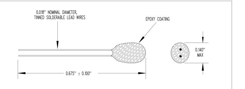
RESISTANCE @  $+25^{\circ}C$  =  $10,000 \Omega \pm 1\%$ RESISTANCE/TEMPERATURE CURVE = "J" BETA " $\beta$ " (0 TO  $+50^{\circ}C$ ) =  $3,892^{\circ}K$  NOMINAL TEMPERATURE COEFFICIENT @  $+25^{\circ}C$  = -4.4%/'C NOMINAL DISSIPATION CONSTANT = 2 mW/°C NOMINAL THERMAL TIME CONSTANT = 15 SECONDS NOMINAL (STILL AIR) THERMAL TIME CONSTANT = 3 SECONDS MAXIMUM (STIRRED OIL) MAXIMUM TEMPERATURE RATING =  $+125^{\circ}C$
