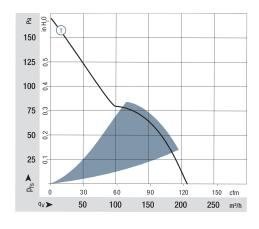
Air performance measured according to: ISO 5801. Installation category A, without contact protection. Noise: Total sound power level  $L_WA$  ISO 103002 measured on a hemisphere with a radius of 2 m. Sound pressure level  $L_PA$  measured at 1 m distance from fan axis. The values given are applicable only under the specified
