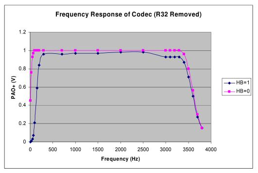
As can be seen from the chart, the codec frequency response is flat between 300 and 3,300 Hz. With the high pass filter on, the 3dB points are at 150Hz and 3,600 Hz respectively. With the high pass filter off, the 3dB point goes down to approximately 15Hz.
