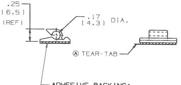
ADHESIVE BACKING: PRESSURE SENSITIVE FOAM TAPE, .04(1.0) THICK, WITH RUBBER (-A)ACRYLIC (-AT) OR HIGH BOND ACRYLIC (-AV) ADHESIVE AND PROTECTIVE LINER. LINER TO EXTEND BEYOND EDGE TO FORM TEAR-TAB. MOUNT IS DESIGNED TO SUPPORT .20 lbs. (91g) MAX. WEIGHT ON A CLEAN, DRY, SMOOTH SURFACE,
