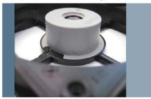
"U" version (optional) IP65 ingress protection rating with VDE certificate (full encapsulation of winding and PCB)
