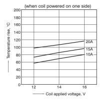
1.-(2) Coil temperature rise (at 85°C 185°F) Sample: ACJ1212, 3pcs Measured portion: Inside the coil
