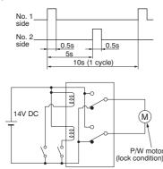
Load current waveform Current value: 25A
