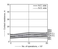
5.-(2) Electrical life test (Motor lock)
