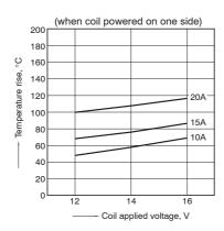
1.-(5) Coil temperature rise (at room temperature)
