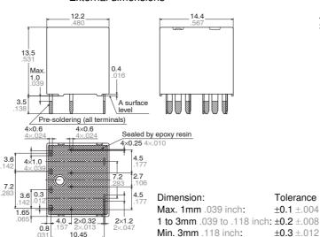
Dimensions (thickness and width) of terminal is measured before pre-soldering Intervals between terminals is measured at A surface level.
