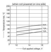
1.-(3) Coil temperature rise (at room temperature)
