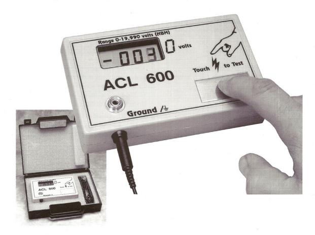
The ACL 600 is a new and unique visual method of detecting how much static charge a person is carrying. The unit can be easily wall mounted outside the ESD protected area to avoid charged persons unknowingly entering. Operators also find this unit useful to periodically check that they are not creating a charge within the protected area.
