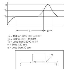
Cautions for mounting operations Temperature profile indicates the temperature of the soldered part (\*1) of terminals on the surface of a circuit board. The exterior temperature of a relay may be extremely high depending on the component density on the board or the heating method of the reflow oven or circuit board type. Sufficient verification under actual processing conditions is required.
