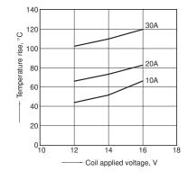
1-(2). Coil temperature rise Sample: ACNM7112, 3pcs Measured portion: Inside the coil Contact carrying current: 10A, 20A Ambient temperature: 110°C 230°F
