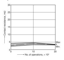
5-(3). Electrical life test (Lamp load) Sample: ACNM3112, 3pcs. Load: inrush: 84A/steady: 12A Switching frequency: (ON:OFF = 1s:14s) Ambient temperature: Room temperature
