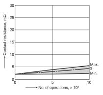
5-(2). Electrical life test (Motor load) Sample: ACNM7112, 3pcs. Load: inrush: 80A/steady: 16A, radiator fan actual load (motor free) Switching frequency: (ON:OFF = 2s:6s) Ambient temperature: 110°C 230°F
