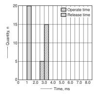
5-(1). Electrical life test (Resistive load) Sample: ACNM1112, 3pcs. Load: Resistive load (NO side: 30A 14V DC) Operating frequency: (ON:OFF = 1s:1s) Ambient temperature: Room temperature
