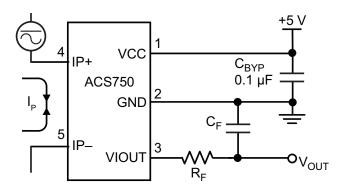
Application 1. The ACS750 outputs an analog signal,  $V_{OUT}$ . that varies linearly with the uni- or bi-directional AC or DC primary sensed current,  $I_P$ , within the range specified.  $C_F$  is recommended for noise management, with values that depend on the application.
