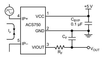
Application 1. The ACS750 outputs an analog signal,  $V_{OUT}$ . that varies linearly with the uni- or bi-directional AC or DC primary sampled current,  $I_P$ , within the range specified.  $C_F$  is recommended for noise management, with values that depend on the application.
