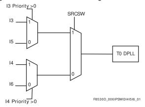
When external protection switching is enabled, the device will operate as a simple switch. All clock monitoring is disabled and the DPLL will simply be forced to try to lock on to the indicated reference source. Consequently the device will always indicate "locked" state in the  $sts\_operating$  register (Reg. 09, Bits [2:0]).
