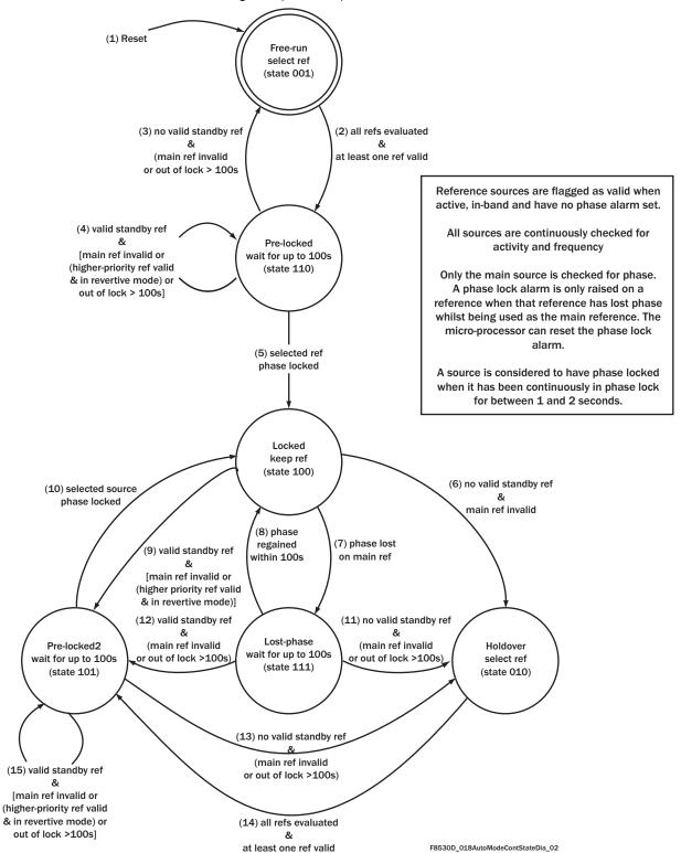
Note... The state diagram above is for TO DPLL only, and the 3-bit state value refers to the register sts\_operating Reg. 09 Bits [2:0] TO\_DPLL\_operating \_mode. By contrast, the T4 DPLL has only automatic operation and can be in one of only two possible states: "Instantaneous Automatic Holdover" with zero frequency offset (its start-up state), or "Locked". The T4 DPLL states are not configurable by the User and there is no "Free-run" state.
