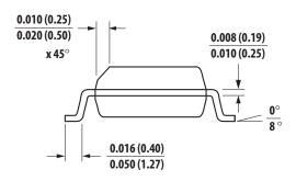
DIMENSIONS: INCHES (MILLIMETERS)  $\frac{MIN}{MAX}$
