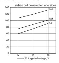
1-(2). Coil temperature rise (at 85°C 185°F) Sample: ACT212, 3pcs. Contact carrying current: 0A, 10A, 20A Ambient temperature: 85°C 185°F
