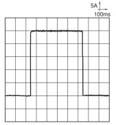
6-(3). Electrical life test (Motor lock) Sample: ACT212, 3pcs. Load: 20A 14V DC,
