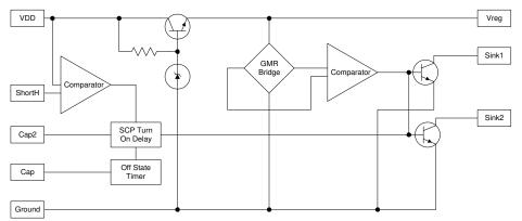
These digital sensors with SCP are available for use with current sinking or current sourcing outputs, in a range of magnetic field operate points. They are provided in an
