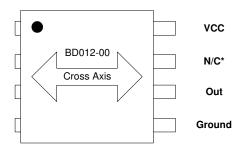
The maximum length of the clipped leads is 0.30mm, leading to an overall package length of 4.25mm, as compared to 4.90mm for the normal MSOP8 package. This part is available in tape and reel format only.
