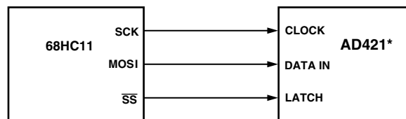
Figure 8. AD421 to 68HC11 Interface
