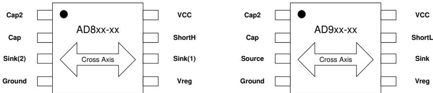
Pin configuration and sensitivity direction for the AD0xx-10 TDFN6 package are defined in the drawing below:
