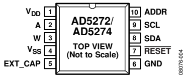
Figure 4. MSOP Pin Configuration
