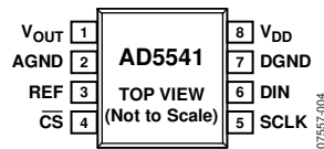
Figure 4. AD5541 Pin Configuration
