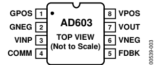
Figure 3. 8-Lead CERDIP Pin Configuration
