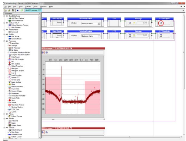
Figure 16. VisualAnalog – [Canvas – (AD6657 FFT)*] Main Window – Showing AD6657 Average FFT Analysis
