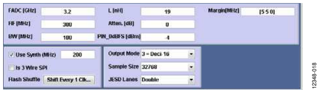
Figure 66. Screenshot of AD6676 GUI Software Tool that Facilitates Device Configuration and Evaluation
