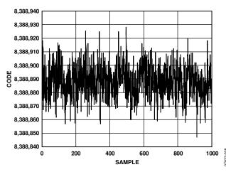
Figure 8. Noise ( $V_{REF} = AV_{DD} = 5 V$ , Output Data Rate = 2400 Hz, Gain = 1, Chop Disabled, Sinc<sup>4</sup> Filter)
