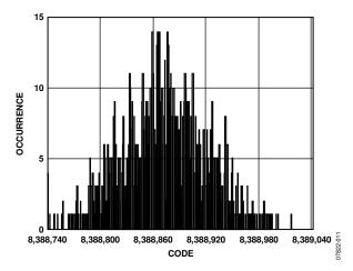
Figure 11. Noise Distribution Histogram ( $V_{REF} = AV_{DD} = 5 V$ , Output Data Rate = 2400 Hz, Gain = 128, Chop Disabled, Sinc<sup>4</sup> Filter)
