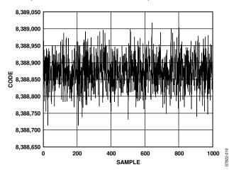
Figure 10. Noise ( $V_{REF} = AV_{DD} = 5 V$ , Output Data Rate = 2400 Hz, Gain = 128, Chop Disabled, Sinc<sup>4</sup> Filter)
