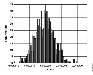
Figure 9. Noise Distribution Histogram ( $V_{REF} = AV_{DD} = 5 V$ , Output Data Rate = 2400 Hz, Gain = 1, Chop Disabled, Sinc<sup>4</sup> Filter)
