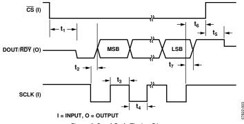
Figure 3. Read Cycle Timing Diagram
