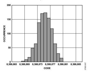
Figure 7. Noise Distribution Histogram ( $V_{REF} = AV_{DD} = 5 V$ , Output Data Rate = 4.7 Hz, Gain = 128, Chop Disabled, Sinc<sup>4</sup> Filter)
