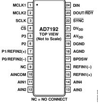
Figure 5. Pin Configuration
