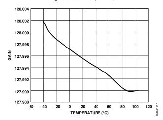
Figure 17. Gain Error (Gain = 128)
