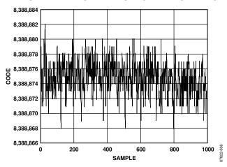
Figure 6. Noise ( $V_{REF} = AV_{DD} = 5 V$ , Output Data Rate = 4.7 Hz, Gain = 128, Chop Disabled, Sinc<sup>4</sup> Filter)
