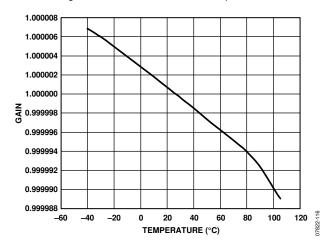
Figure 16. Gain Error (Gain = 1)
