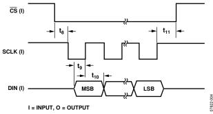
Figure 4. Write Cycle Timing Diagram
