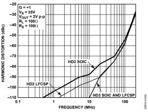
Figure 19. Harmonic Distortion vs. Frequency for Various Packages
