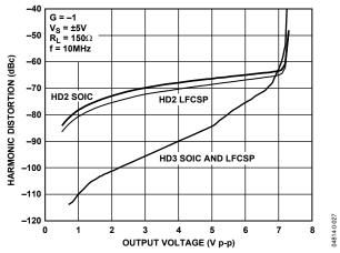
Figure 27. Harmonic Distortion vs. Output Voltage
