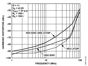
Figure 29. Harmonic Distortion vs. Frequency for Various Packages
