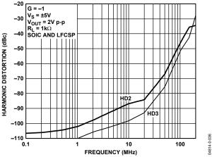
Figure 20. Harmonic Distortion vs. Frequency for Various Packages
