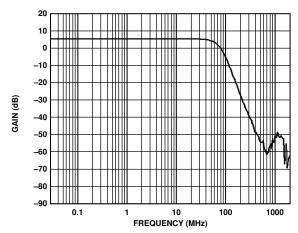
Figure 70. 90 MHz Low-Pass Filter Response
