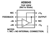
Figure 1. 8-Lead AD8045 LFCSP (CP-8)
