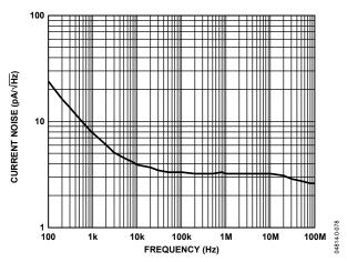
Figure 45. Current Noise vs. Frequency
