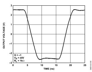
Figure 41. Large Signal Transient Response, Inverting
