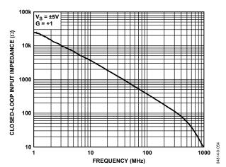
Figure 48. Input Impedance vs. Frequency
