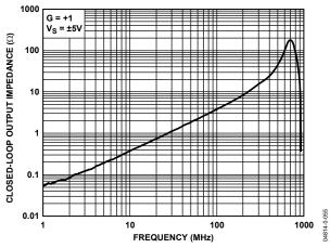
Figure 49. Output Impedance vs. Frequency
