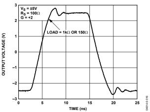
Figure 38. Large Signal Transient Response for Various Loads
