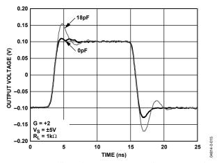
Figure 37. Small Signal Transient Response with Capacitive Load
