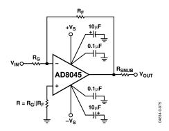
Figure 62. Inverting Configuration
