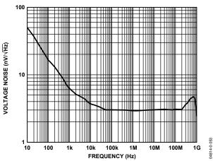
Figure 44. Voltage Noise vs. Frequency
