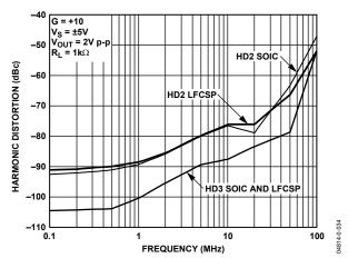
Figure 23. Harmonic Distortion vs. Frequency for Various Packages
