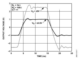
Figure 39. Large Signal Transient Response for Various Supplies
