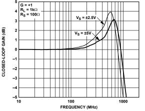
Figure 9. Small Signal Frequency Response for Various Supplies
