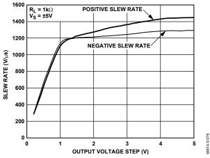
Figure 33. Slew Rate vs. Output Voltage
