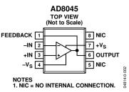
Figure 2. 8-Lead AD8045 SOIC/EP (RD-8)
