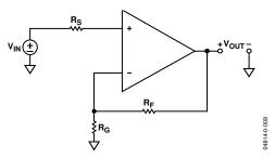
Figure 64. Noninverting Configuration
