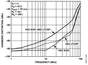
Figure 28. Harmonic Distortion vs. Frequency for Various Packages
