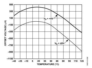
Figure 54. Offset Voltage vs. Temperature for Various Supplies
