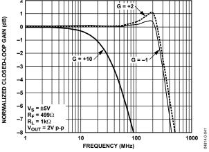
Figure 15. Large Signal Frequency Response for Various Gains
