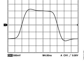
Figure 71. Small Signal Transient Response of 90 MHz LPF
