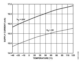
Figure 57. Supply Current vs. Temperature for Various Supplies
