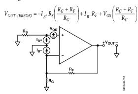
Figure 65. Amplifier DC Errors
