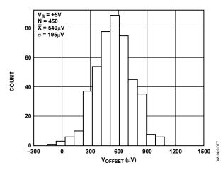
Figure 53.  $V_{OS}$  Distribution for  $V_S = +5 V$
