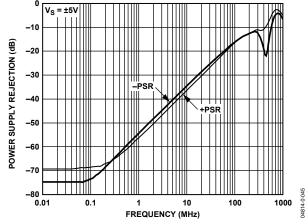
Figure 46. Power Supply Rejection vs. Frequency
