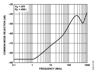
Figure 47. Common-Mode Rejection vs. Frequency
