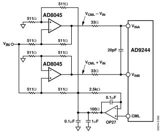
Figure 67. High Speed ADC Driver
