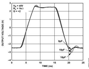
Figure 40. Large Signal Transient Response with Capacitive Load
