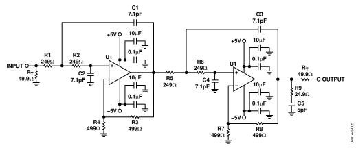
Figure 73. 4-Pole, 90 MHz, Sallen-Key Low-Pass Filter
