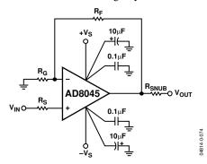
Figure 61. Noninverting Configuration
