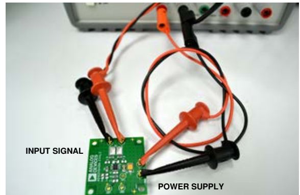
Figure 4. AD8209A Evaluation Board with the Source Signal Connected
