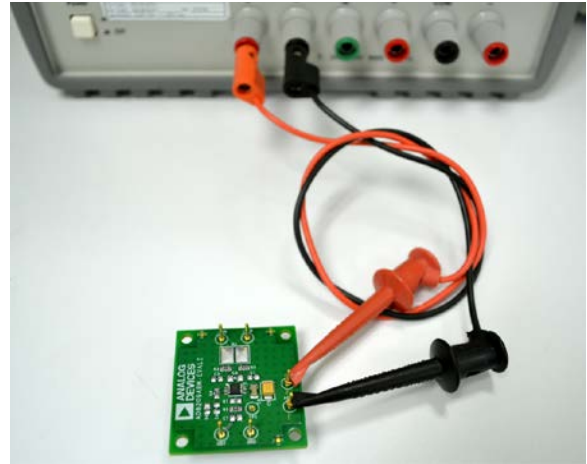
Figure 3. Basic Power Connections of the AD8209A Evaluation Board
