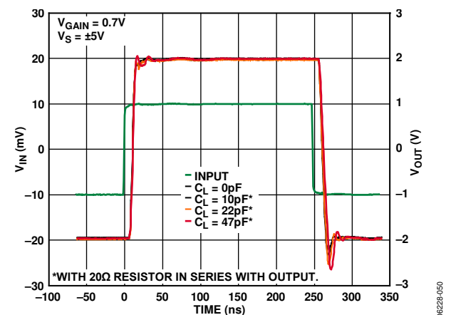
Figure 50. Large-Signal Pulse Response for Various Values of Load Capacitance Using \pm 5 V Power Supplies (See Figure 65)
