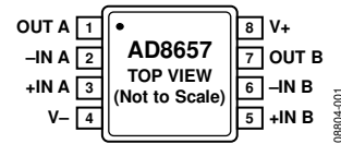
Figure 1. AD8657 Pin Configuration, 8-Lead MSOP
