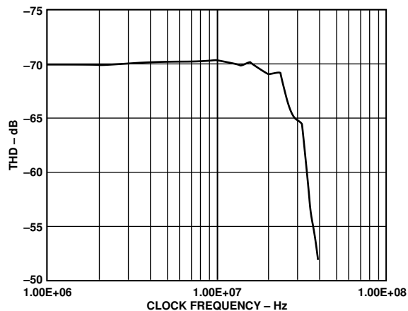
Figure 9. THD vs. Clock Frequency ( f_{IN} = 1 \text{ MHz} )
