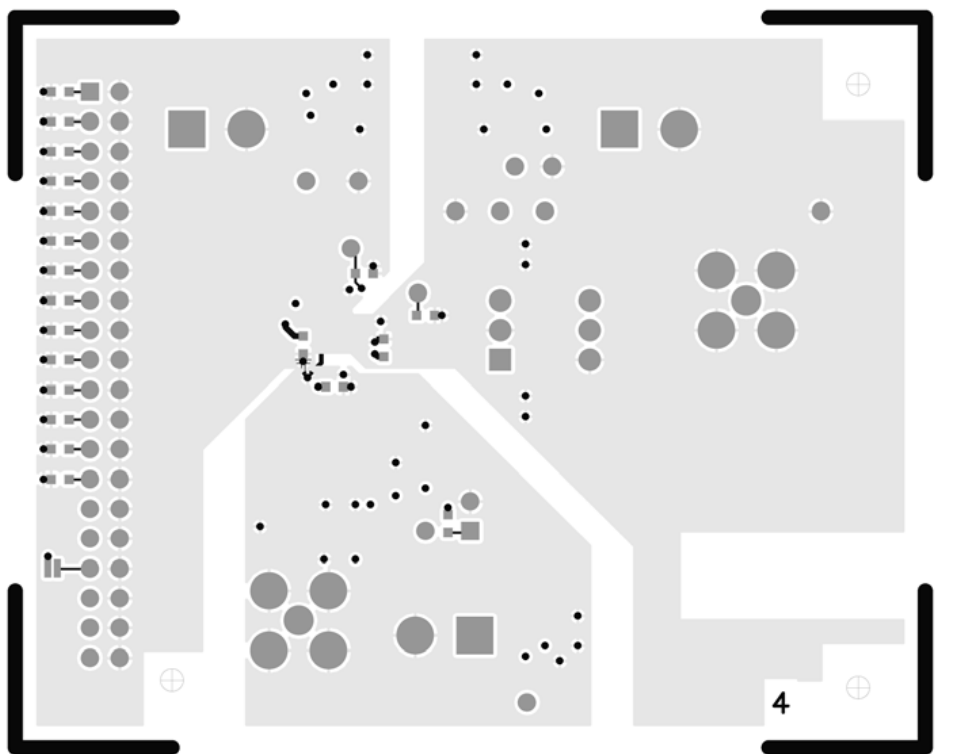
Figure 36. Evaluation Board Layout—Secondary Side
