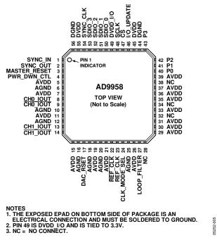
Figure 3. Pin Configuration
