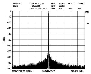
Figure 14. NBSFDR,  $f_{OUT} = 75.1$  MHz,  $f_{CLK} = 500$  MSPS,  $\pm 1$  MHz
