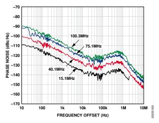
Figure 18. Residual Phase Noise (SSB) with  $f_{OUT}$  = 15.1 MHz, 40.1MHz, 75.1 MHz,100.3 MHz;  $f_{CLK}$  = 500 MHz with REFCLK Multiplier = 20×
