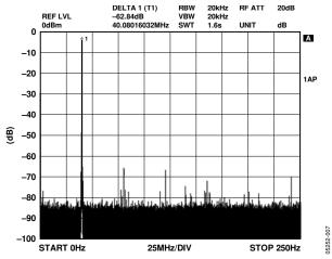
Figure 5. Wideband SFDR,  $f_{OUT} = 40.1$  MHz,  $f_{CLK} = 500$  MSPS
