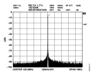
Figure 12. NBSFDR,  $f_{OUT} = 100.3$  MHz,  $f_{CLK} = 500$  MSPS,  $\pm 1$  MHz
