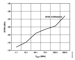
Figure 21. Averaged Channel SFDR vs. fout
