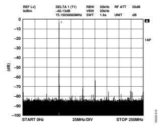
Figure 8. Wideband SFDR,  $f_{OUT} = 75.1$  MHz,  $f_{CLK} = 500$  MSPS
