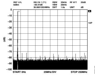
Figure 7. Wideband SFDR,  $f_{OUT} = 15.1 \text{ MHz}$ ,  $f_{CLK} = 500 \text{ MSPS}$
