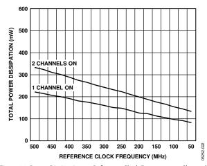
Figure 20. Power Dissipation vs. Reference Clock Frequency vs. Channel(s)
