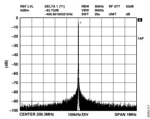
Figure 15. NBSFDR  $f_{OUT}$  = 200. 3MHz,  $f_{CLK}$  = 500 MSPS, , ±1 MHz
