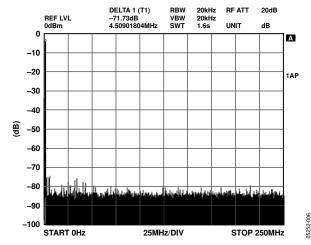
Figure 4. Wideband SFDR,  $f_{OUT} = 1.1 \text{ MHz}$ ,  $f_{CLK} = 500 \text{ MSPS}$
