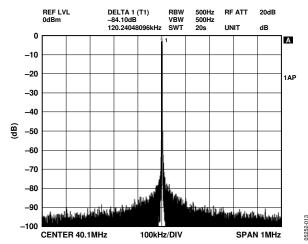
Figure 11. NBSFDR,  $f_{OUT} = 40.1$  MHz,  $f_{CLK} = 500$  MSPS,  $\pm 1$  MHz
