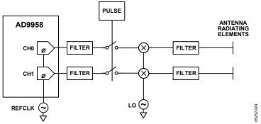
Figure 22. Phase Array Radar Using Precision Frequency/Phase Control from DDS in FMCW or Pulsed Radar Applications;
