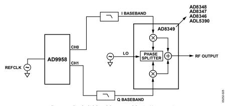
Figure 23. Single-Sideband-Suppressed Carrier Upconversion
