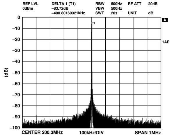
Figure 15. NBSFDR  $f_{OUT} = 200.3$  MHz,  $f_{CLK} = 500$  MSPS,  $\pm 1$  MHz
