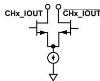
TERMINATE OUTPUTS INTO AVDD. DO NOT EXCEED VOLTAGE COMPLIANCE OF OUTPUTS.
