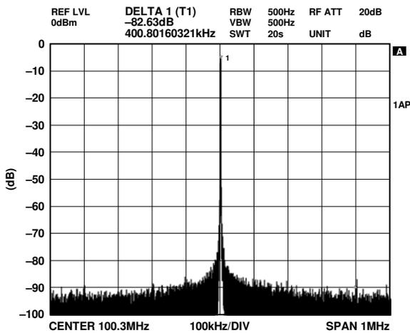
Figure 12. NBSFDR,  $f_{OUT} = 100.3$  MHz,  $f_{CLK} = 500$  MSPS,  $\pm 1$  MHz
