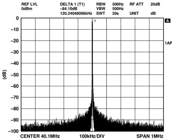
Figure 11. NBSFDR,  $f_{OUT} = 40.1$  MHz,  $f_{CLK} = 500$  MSPS,  $\pm 1$  MHz
