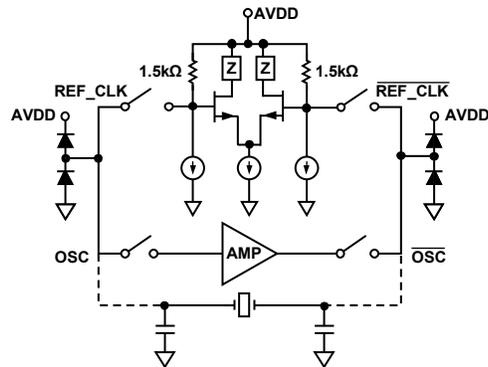
REF\_CLK INPUTS ARE INTERNALLY BIASED AND NEED TO BE AC-COUPLED. OSC INPUTS ARE DC-COUPLED.
