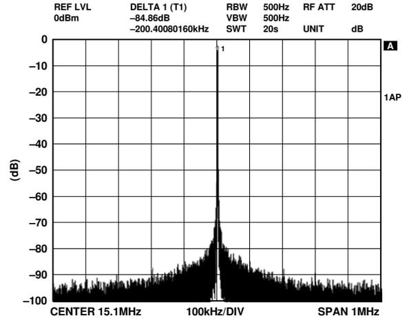
Figure 13. NBSFDR,  $f_{OUT} = 15.1$  MHz,  $f_{CLK} = 500$  MSPS,  $\pm 1$  MHz
