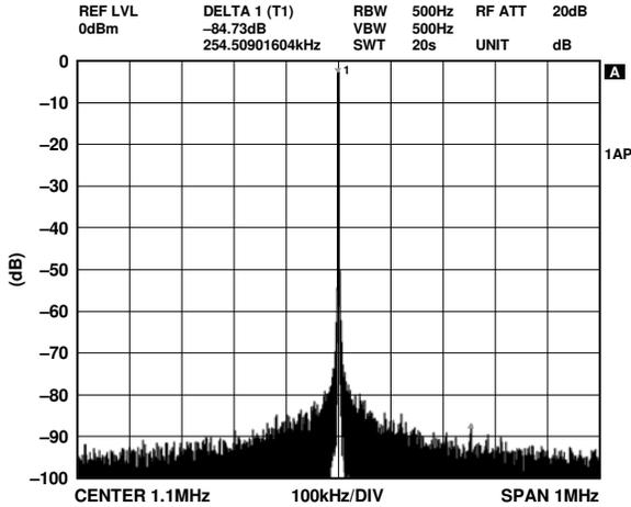
Figure 10. NBSFDR,  $f_{OUT} = 1.1$  MHz,  $f_{CLK} = 500$  MSPS,  $\pm 1$  MHz
