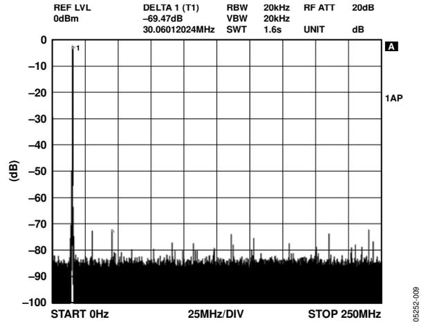
Figure 7. Wideband SFDR,  $f_{OUT} = 15.1$  MHz,  $f_{CLK} = 500$  MSPS
