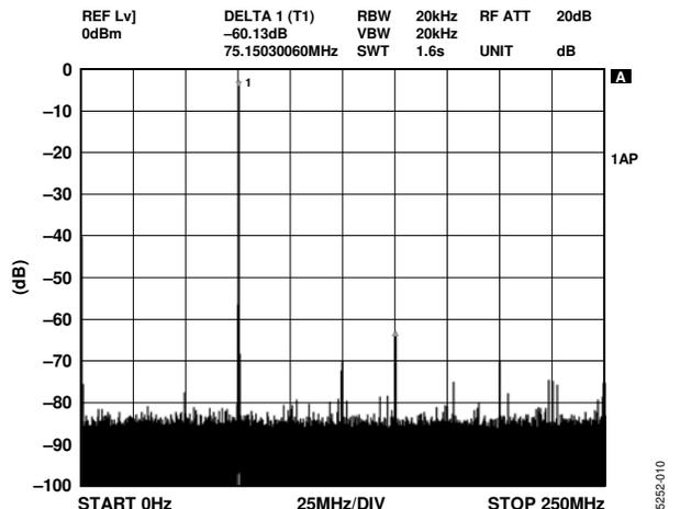
Figure 8. Wideband SFDR,  $f_{OUT} = 75.1$  MHz,  $f_{CLK} = 500$  MSPS
