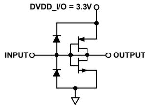
AVOID OVERDRIVING DIGITAL INPUTS. FORWARD BIASING DIODES MAY COUPLE DIGITAL NOISE ON POWER PINS.
