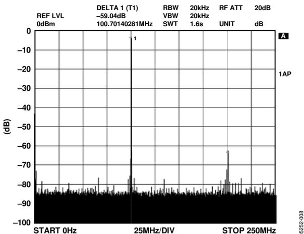
Figure 6. Wideband SFDR,  $f_{OUT} = 100.3$  MHz,  $f_{CLK} = 500$  MSPS
