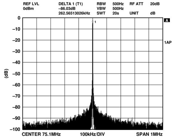
Figure 14. NBSFDR,  $f_{OUT} = 75.1$  MHz,  $f_{CLK} = 500$  MSPS,  $\pm 1$  MHz
