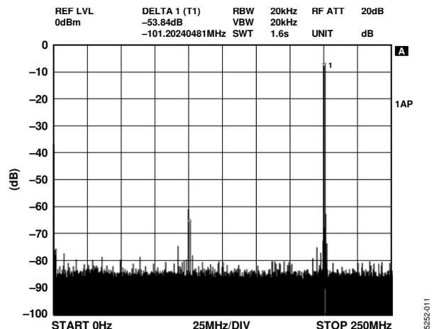
Figure 9. Wideband SFDR,  $f_{OUT} = 200.3$  MHz,  $f_{CLK} = 500$  MSPS
