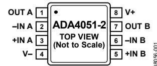
Figure 3. 8-Lead MSOP (RM-8)
