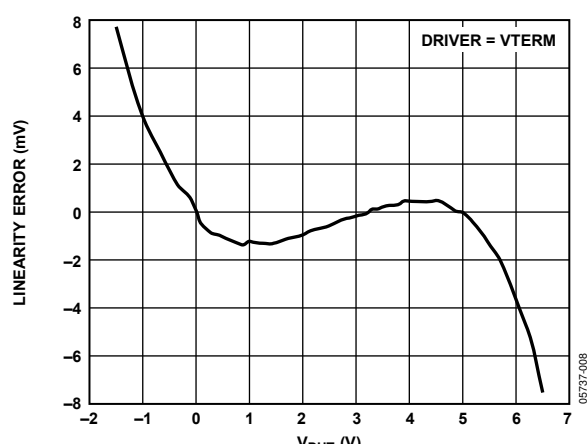
Figure 8. Driver VTERM Linearity vs. Output
